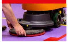
Attach the red pad underneath the scrubbing/suction machine.
