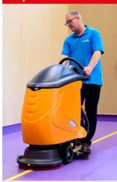
Apply the fluid while scrubbing and let the machine suck it up immediately. Work at a normal walking pace.
