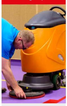
Attach the red pad underneath the scrubbing/suction machine.
